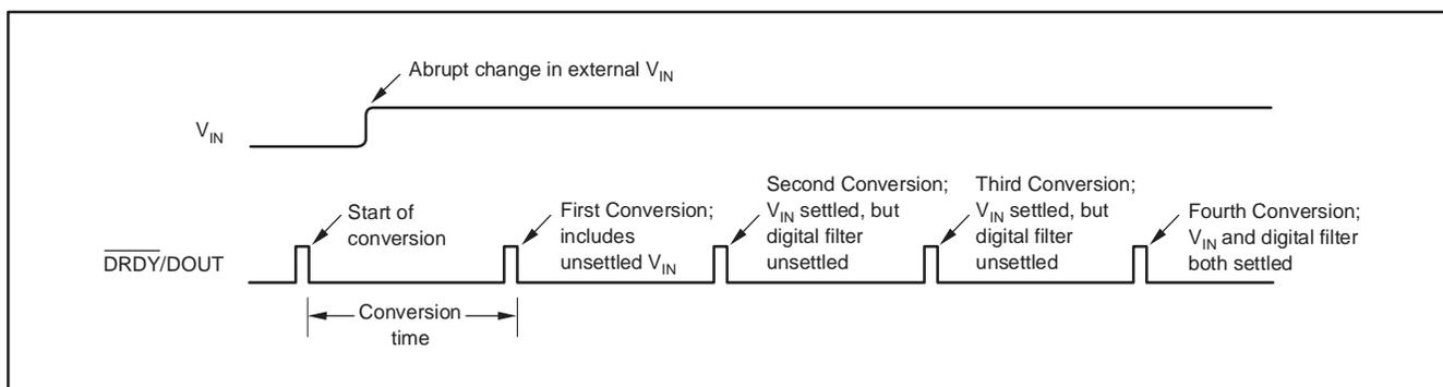
**Figure 24. Settling Time in Continuous Conversion Mode**
