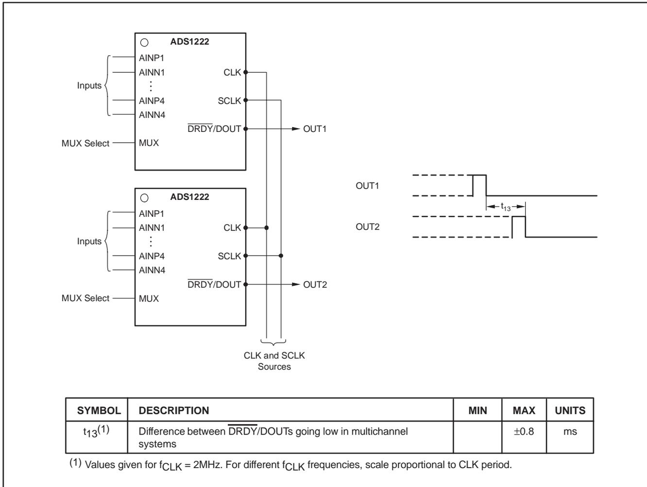
Figure 31. Example of Using Multiple ADS1222s in Parallel
