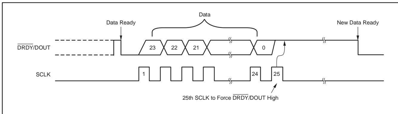
Figure 26. Data Retrieval with  $\overline{\text{DRDY}}/\text{DOUT}$  Forced High Afterwards
