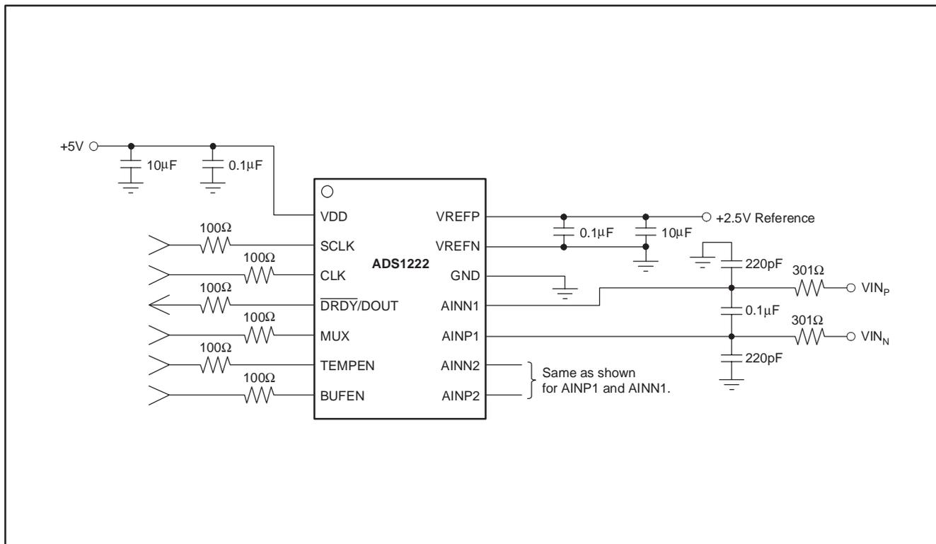
Figure 30. Basic Connections
