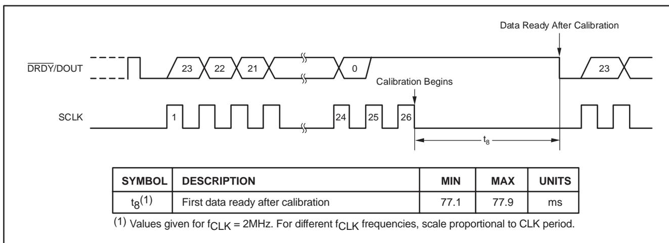
Figure 27. Self-Calibration Timing
