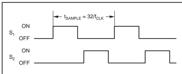
Figure 15.  $S_1$  and  $S_2$  Switch Timing for Figure 14
